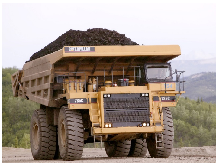
One of UCM's eight 150-ton capacity haul trucks.
